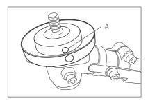
Rotate the gear box shaft until the hole in the holder A lines up with the slot in the metal quard.
