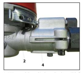
5. Ensure the locking pin (4) is securely located in the angle selector (2) before using.
