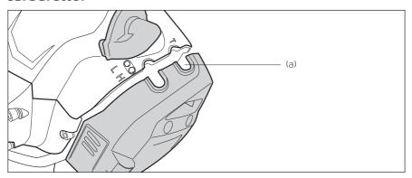
The carburettor mixture setting has been set at the factory and will not need adjusting. **Adjusting the idle speed:** If adjustment is necessary turn the T screw (a) clockwise until the cutting head starts to move, then turn the T screw anticlockwise until the cutting head stops. **If the idle speed cannot be adjusted to stop the cutting head moving at idle, contact your dealer for repair before use.**
