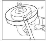
Insert an Allen key or screwdriver into the hole in the gearbox cover and into holder A.
