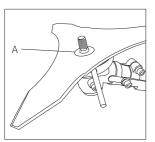
Place the 3 tooth blade on the holder A, centering the blade on the raised centre.
