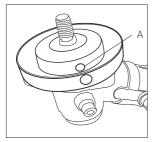
Rotate the gear box shaft until the hole in the holder A lines up with the slot in the metal guard.
