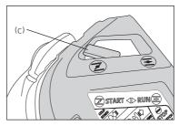
Fig 2 - Move the choke lever (c) to the START ( \) position.
