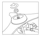
Fit the nut anti-clockwise (turn left) and tighten using the spanner provided. Remove the Allen key / screwdriver.
