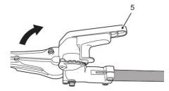
**6.** Release the red locking lever and ensure the locking pin engages with the quadrant.
