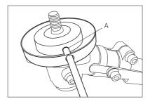
Insert an Allen key or screwdriver into the hole in the gearbox cover and into holder A.
