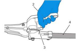
**5.** While holding the shaft (4), move the cutting head to the desired position.
