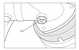
Remove the bolt (a) on the gear case, top up the gearbox using Lithium grease and refit the bolt.
