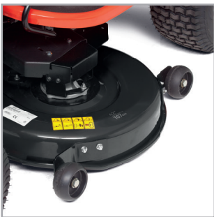
FRAME HUNG MOWER DECK With 4 deck support wheels and a washout port for easy cleaning.
