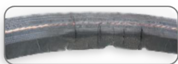
Cracked underside of belt
