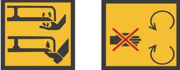
Do not place hands or feet under cutting deck. Do not touch rotating parts.
