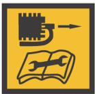
Stop the engine and remove the spark plug wire before assembly, maintenance and unblocking debris.
