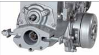
Two power take-offs, one independent two-speed PTO and one synchronised PTO.
