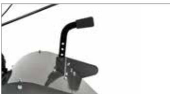
50 cm cutter with depth regulator.
