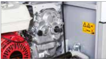
Independent PTO at 2100 rpm.
