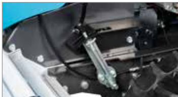
Direct engagement gear lever.
