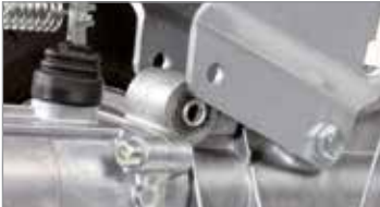
Handlebar mounted on vibration dampers.
