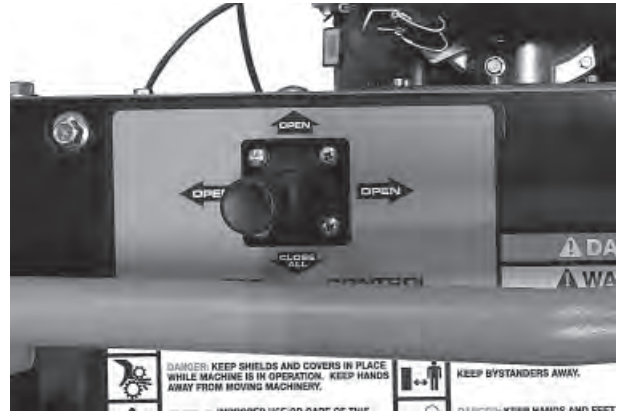
Deflector Control Switches
