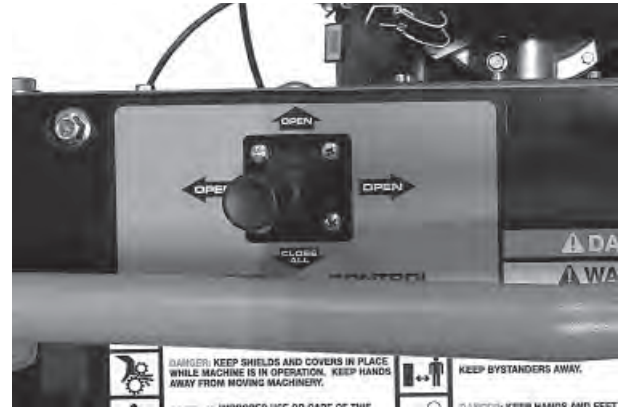
Deflector Control Switches
