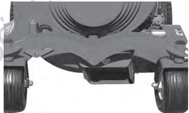
Front Discharge Chute
