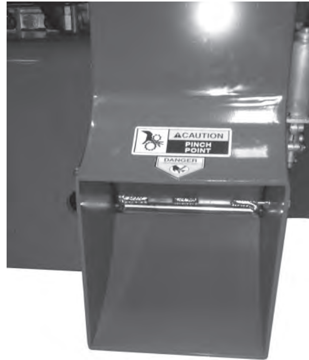
Right Discharge Chute
