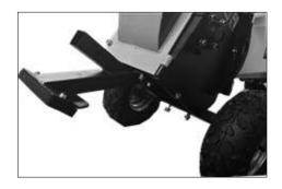
4. Fit the front resting plate. Secure the front support with the bolts provided.
