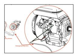
8. Attach the emergency stop wire. Before operating fit the emergency stop wire. Check the engine stops correctly before operating in every case.
