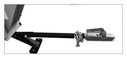
6. Fit the tow bar to the front resting plate with the bolts provided, fully tighten and ensure securely fitted.
