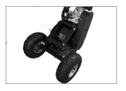
1. Remove from packing & fitting the wheel axle. Use a block to support whilst securing and fitting the axle for the transport wheels.
