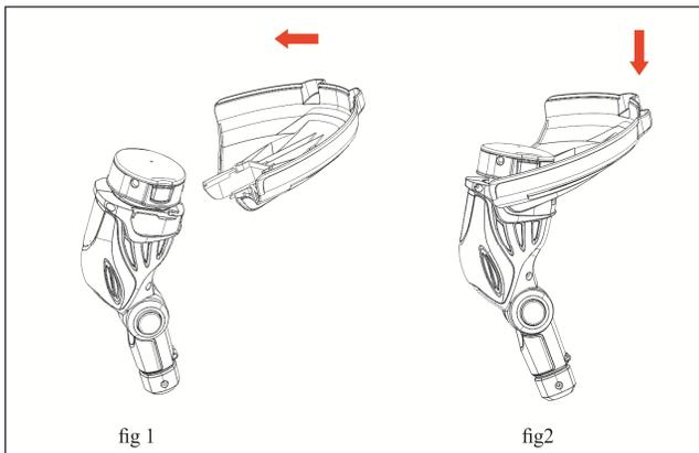
Insert the locating support of the guard into the trimmer head as shown in figure1 above, carefully push the guard down, see figure 2, so that it locks in place.
