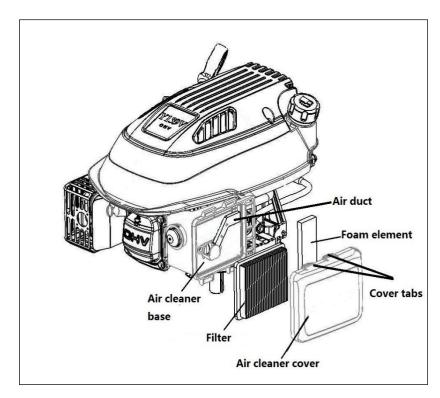
NOTE: Replace filter if frayed, torn, damaged or unable to be cleaned.
