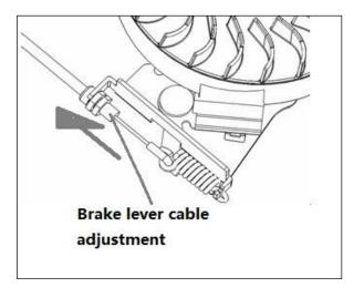
Engine brake adjustment:
