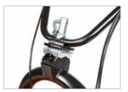
Handlebar with vertical and horizontal adjustment using the handlebar-mounted lever.
