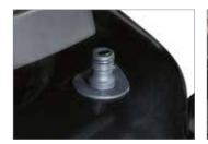
The quick-fit "Deck Wash System" connector on the mowing deck makes it possible to direct water inside the deck for quick and easy cleaning of the cutting mechanism (106).
