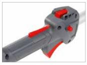
AlwaysOn system: the ON/OFF switch automatically returns to the ON position after each stop, avoiding the risk of engine flooding.
