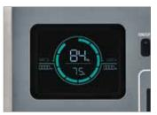
The display shows various information such as remaining charge status, instantaneous load, or input charging power.
