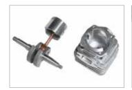
Piston with 2 elastic rings, forged and machined steel crankshaft and connecting rod, needle roller bearings, nickel plated cylinder: constant high efficiency guaranteed over time, even when undertaking heavy work schedules.
