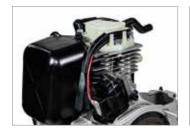
Engine with 4-stroke technology and overhead valves (OHV).
