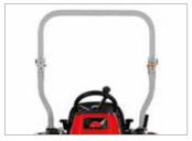
Equipped as standard with roll bar, front and rear bumpers, side guards and seat belt to ensure maximum safety, even when tackling the most complex situations (TONKAWA).
