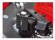
**TKE** models with Emak engine and rechargeable battery-powered electric starting ensure effortless starting every time. The engine is also equipped with recoil starter.
