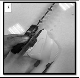
To seat the blade housing, press both blade release buttons and press against the main motor housing, until seated and then release both blade release buttons (3 & 4)
