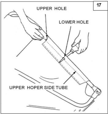
STEP 22 Insert a  $\emptyset$ 8X59.5 clevis pin through the lower hole in each upper hopper side tube. Next assemble a bag arm tube onto each clevis pin and secure it with a hair cotter pin  $\emptyset$ 3.
