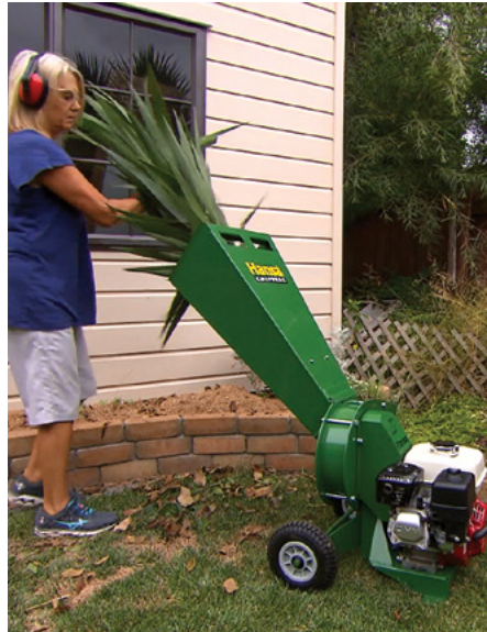
Model C4 in action, one in-feed chute – will handle fibrous material such as palm fronds
