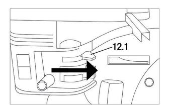
When the engine is running, the speed can be adjusted by moving the throttle control lever (13.1) to the high (indicated by a hare), medium or low position (indicated by a tortoise).
