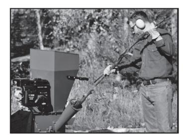
When finished chipping, turn **OFF** the machine, allow all moving parts to come to a complete stop, and disconnect the spark plug wire before moving the machine, emptying the bag, unclogging the inlets or outlets, filling the gas tank, or performing maintenance and repairs.
