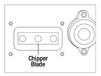
Remove one blade, rotate the impeller, and remove the second blade. Have the original blades professionally sharpened, or order a replacement set, then re-install the blades. Replace the side cover plate and re-attach the spark plug wire.
