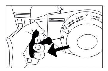
When the engine has been successfully started and is running smoothly return the choke lever to the <u>OFF</u> position (12.1).
