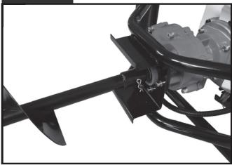
Insert the drive pin. Secure with R-pin.
