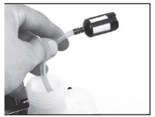
Pull old filter from fuel pipe and replace with new filter.
