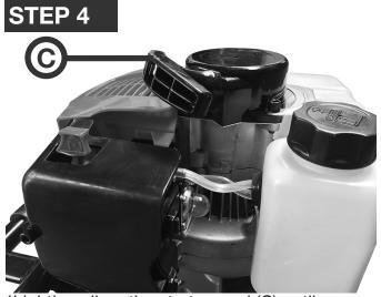
4Lightly pull on the starter cord (C) until you can feel resistance, then pull on the cord quickly and firmly until the engine starts.
