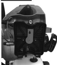
Carefully remove the foam filter insert and check it for damage. Replace if required.
