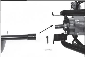
Place the motor casing on a work bench. Place the earth auger on the drive shaft, ensuring that both holes are aligned.
