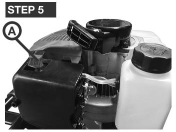
After running for 10 seconds or so, squeeze the throttle trigger to release the choke lever (A) to the RUN position.
