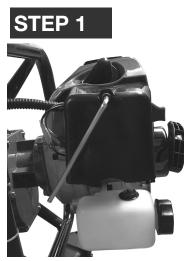
Loosen the screw on the air filter casing. Remove the air filter cover and check it.
