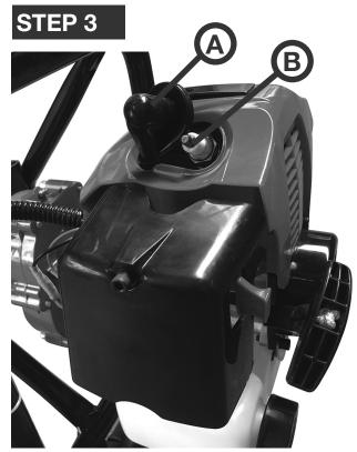
Remove the spark plug cover (A) by removing the screw (B) with the provided key.
