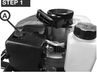
If the engine is cold, move the choke lever (A) to the START position. The choke lever opens and closes the choke in the carburettor.
