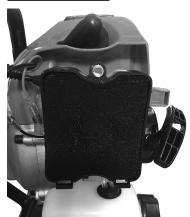
Clean dirt from the inside of the filter casing with a clean, damp cloth.
