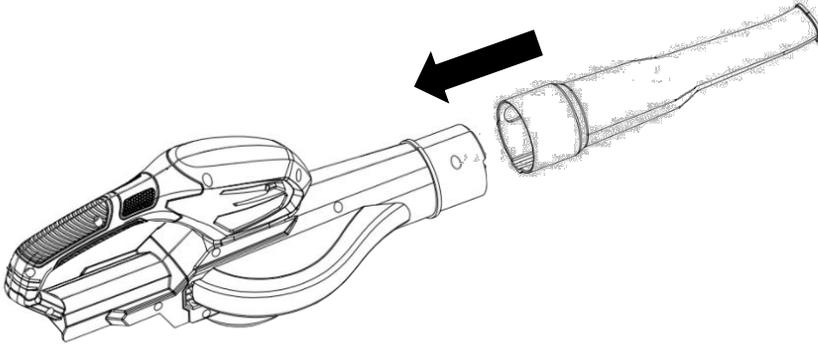
**NOTE –** To remove the **Blower Pipe (C)**, press in the clip and pull away from **Main Body (A)**.
