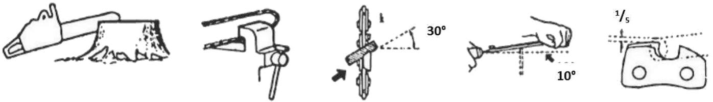
**9.36** After every cutter has been set, check the depth gauge and file to the proper level as illustrated
