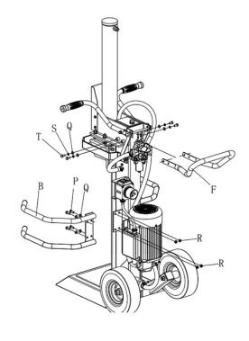
**(h)** Attach all the *HOSES* to the machine as the following, including *HIGH PRESSURE OIL B.*
