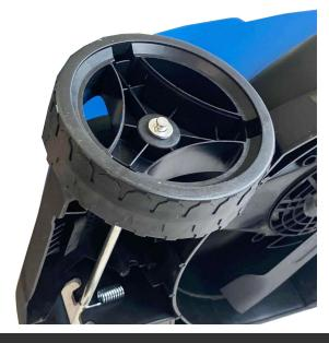
3 Place a split pin through the axle hole. You must spread the split pin after inserting it. This will stop the wheel from falling off.
