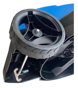
2 You should only have the 4 washers with the large holes left over. Place one over the axle.
