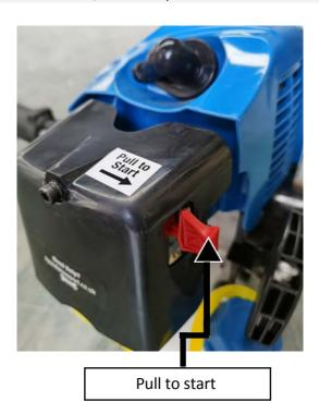
Place one hand on the machine, and using the other hand pull the recoil until you feel a resistance, then pull briskly. Repeat until machine starts.
