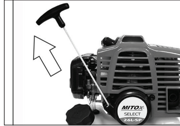
Fig 6 - Pull the starter rope until the engine starts, then squeeze the throttle briefly to release the fast idle control and return the engine to idle.
