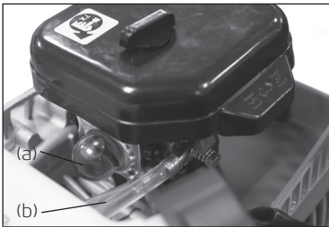
Fig 1 - Push the air purge bulb (a) until fuel is visible in the clear return fuel line (b)
