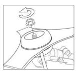
Fit the nut anti-clockwise (turn left) and tighten using the spanner provided. Remove the Allen key / screwdriver.
