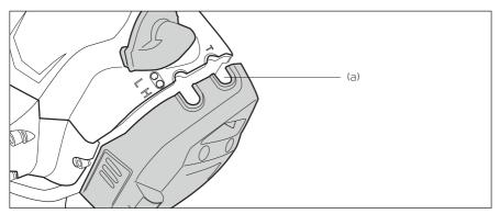
The carburettor mixture setting has been set at the factory and will not need adjusting.
