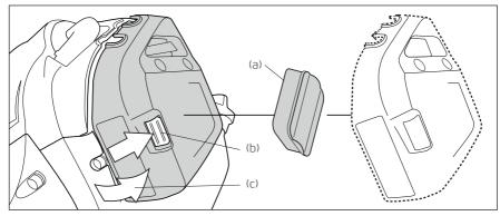
Before using the Pole Pruner, check the air filter (a). Being clogged, will reduce the engine performance. Remove the air filter cover by pressing on the filter cover release (b) and opening the filter cover (c). Clean the filter element in warm, soapy water, dry completely before installing. If the element is broken or shrunk, replace with a new one.
