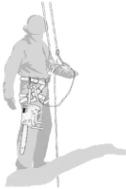
Figure B.1 — Example of attachment of tree service chain-saw to operator's harness
