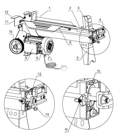
Bleed the air out of the hydraulic system before starting the log splitter. The bleed screw of the hydraulic oil tank should be loosened by three rotations until air can go in and out of the oil tank smoothly. Air flow through the oil tank filler should be detectable during the operation of the log splitter. Before moving the log splitter, make sure the bleed screw is tightened to avoid oil leaking from this point.
