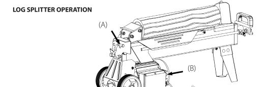
This log splitter is equipped with a control system that requires it to be operated by both hands of the user - Left hand controls the hydraulic control lever (A) while right hand controls the motor control switch (B). The log splitter will stop upon absence of either hand. Only after both hands release the controls, will the log pusher start to return backward to the starting position.
