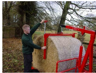
Step 2. Remove the two bale lifting pins
