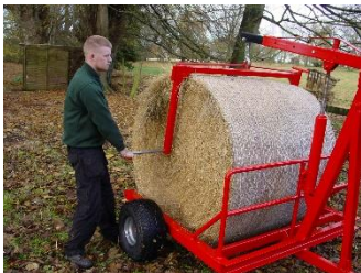
Step 3. Insert the pins into the centre of the bale from both sides
