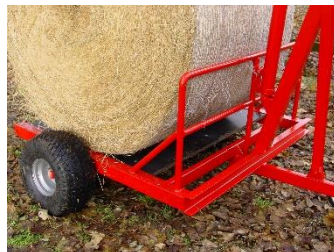
Step 6. Lower bale to floor of trailer before moving
