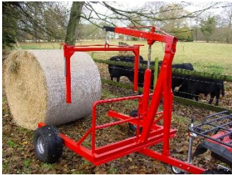
Step 1. With the wooden base removed, reverse carrier to the bale
