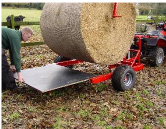
Step 5. Replace the wooden base into frame under bale
