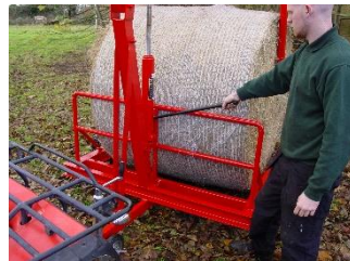
Step 4. Pump the crane to lift the bale
