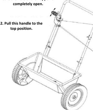
5. Move the position of the nut and change the space between the hole of the hopper and the rotating door.
