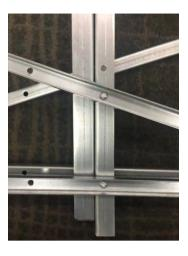
The finished product, should have a large and small section, to allow you to position different length logs for cutting. One section should measure 33cm and the larger section 39.5cm.
