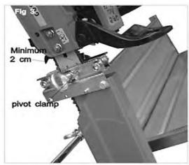
Secure the Saw Guard (14) to the Pivot Clamp, using 8x70mm Bolt & M8 Nut (9). Ensure there is sufficient clearance between the guard and saw chain.
