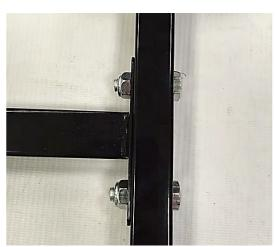
Attach the two Short Legs to the two Long Legs bottom fixing hole, ensuring the L-shape at the top of the Short Leg is positioned on the outside of the Long Leg. Secure using 8x35mm Bolt (2) & M8 Nut (9).
