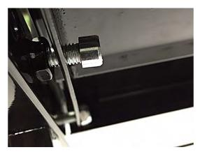
Secure Bed 2 (19) to the Long Leg, using 8x45mm Bolt (3) and M8 Nut (9), into the upper hole of the two located in the leg. The L-shape on the Bed, should sit on the outside of the leg.
