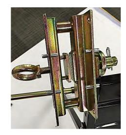
Carefully lower the chainsaw bar into position between the two solid blocks on the pivot clamp and ensure you have a 2cm gap between the body of the chainsaw and the clamp.
