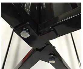
Position the Pivot Clamp Holder (16) into the right-hand Long Leg and secure with the Rod/Handle Eyelet (26) using 10x20mm Bolt (5) & M8 Washer.
