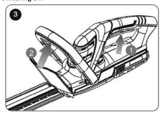
Pull the On/Off trigger upwards with your right hand.
