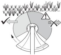
Only cut with the left (shown here as light grey) area of the cutting unit when the unit is being moved from right to left. In the right (dark grey) area, the threads rotate in your direction.
