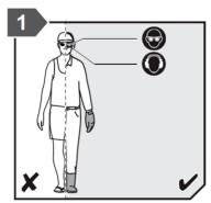
Always wear appropriate footwear, such as work boots, and trousers when operating the mower. Do not operate the equipment
